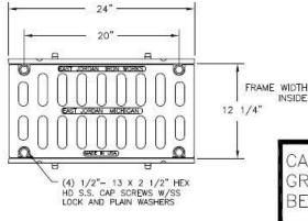
CAUTION: DO NOT DISASSEMBLE BOLTED GRATES AND CHECK <u>FRAME WIDTH INSIDE</u> BEFORE SETTING SECTIONS IN CONCRETE.
